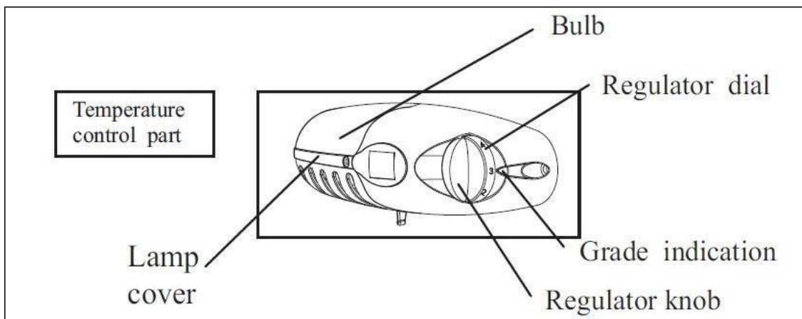
Your appliance has one control for regulating the temperature. The temperature control is located at the top of the device.
